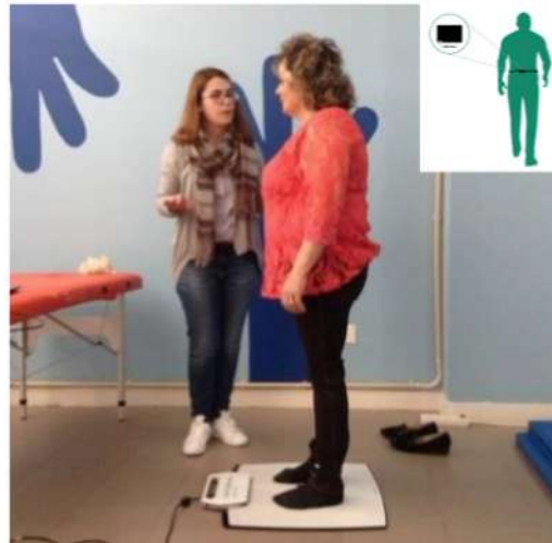
Figure 6.1: Example of a test set-up, with the pressure platform in the floor and an illustration of the inertial sensor placement of at the lower back, since it is covered by the clothes.
