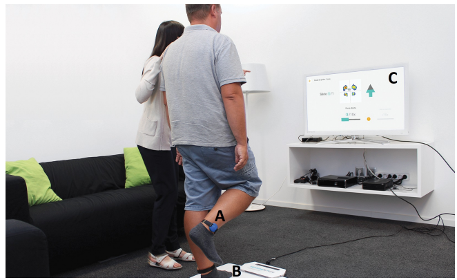
Fig. 1. Healthcare provider and elder interaction with the Clinical Tool during the Knee Flexion exercise. Real-time exercise monitoring using an inertial sensor (A) and a pressure platform (B). Feedback is provided on the screen (C) during the entire exercise, with the current series information, number of performed repetitions, movement phases indication and plantar pressure distributions (heat map).
